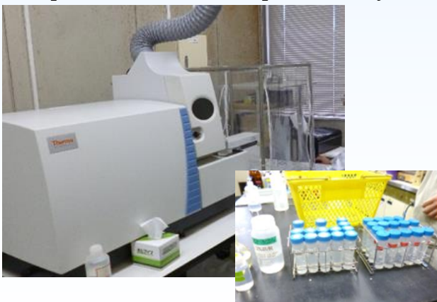
ICP-MSによる重金属の試験 (Analysis of heavy metal by Inductively Coupled Plasma-Mass Spectrometry)
